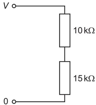
What is the potential difference across the  $10\text{ k}\Omega$  resistor?
